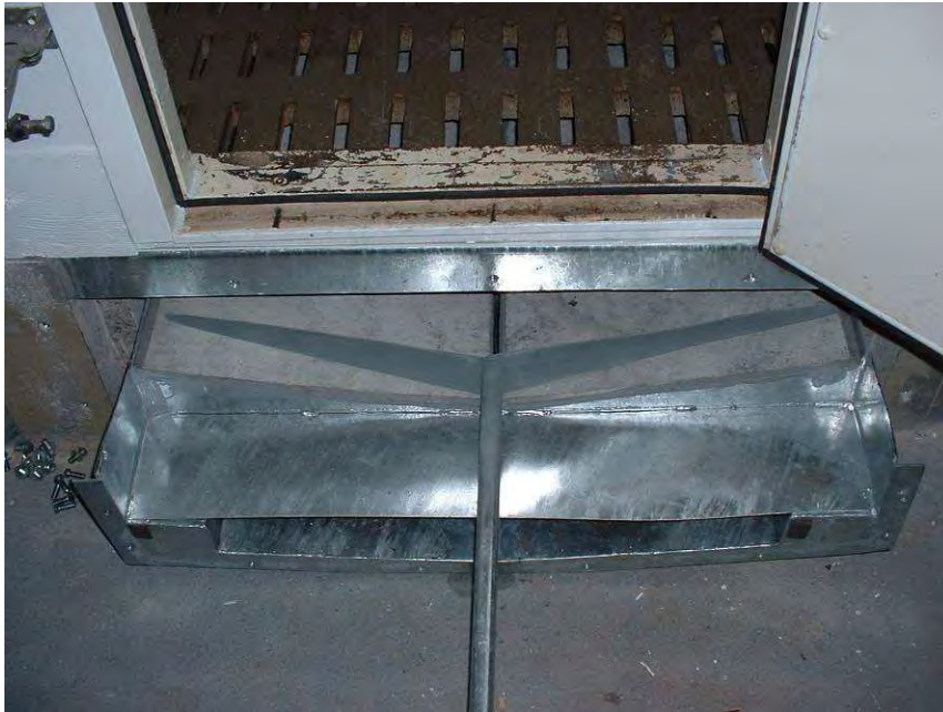
Figure 2. A picture of the V-shape scraper system.
